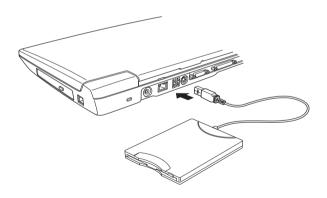
Figure 4-2 Connecting the USB diskette drive
